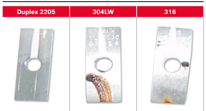
Figure 14: Test coupons half above and half below GeoBrom® HG520 after 90-day exposure at 50 °C before cleaning
