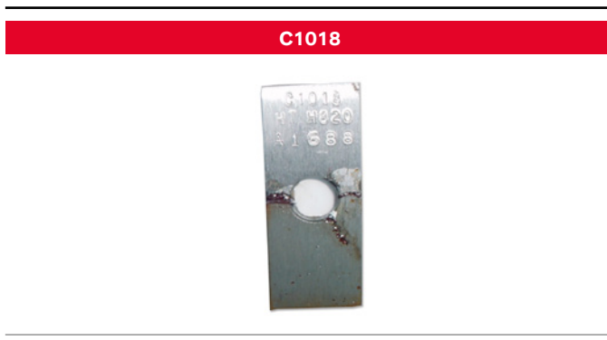
Figure 9: C 1018 coupon at half subsurface before cleaning after 90-day exposure at 20 °C
