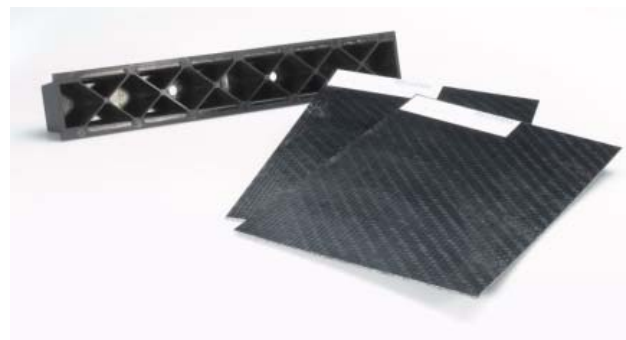
Figure 1 Composite sheets with a test beam
