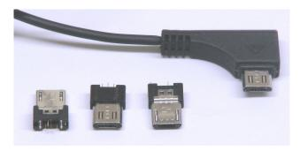
Figure 1 USB connector housings
