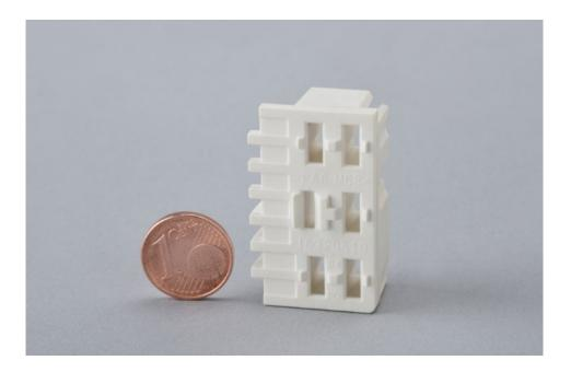
The cooling element of the charge controller for the electric sports car is made of Durethan BTC965FM30. This thermally conductive polyamide 6 prevents overheating during the charging process and meets the strict requirements for flame-retardant properties, tracking resistance and design.
